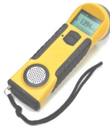
KT-10 v2 Magnetic Susceptibility Meter (Circular Coil)
