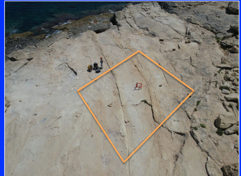
TDEM exploration for groundwater in Malta with 10 m x 10 m TX loop and centrally-located induction coil RX
