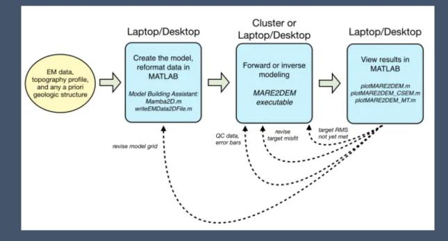
MARE2DEM uses Occam inversion method (Constable et al., 1987) "A practical algorithm for generating smooth models from electromagnetic sounding data"
