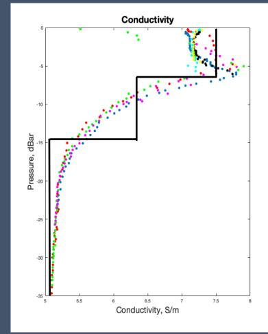
Layers derived from Conductivity-Temperature-Depth (CTD) soundings
