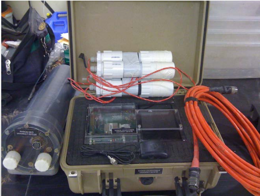
(left) Narod NIMS transportable configuration
