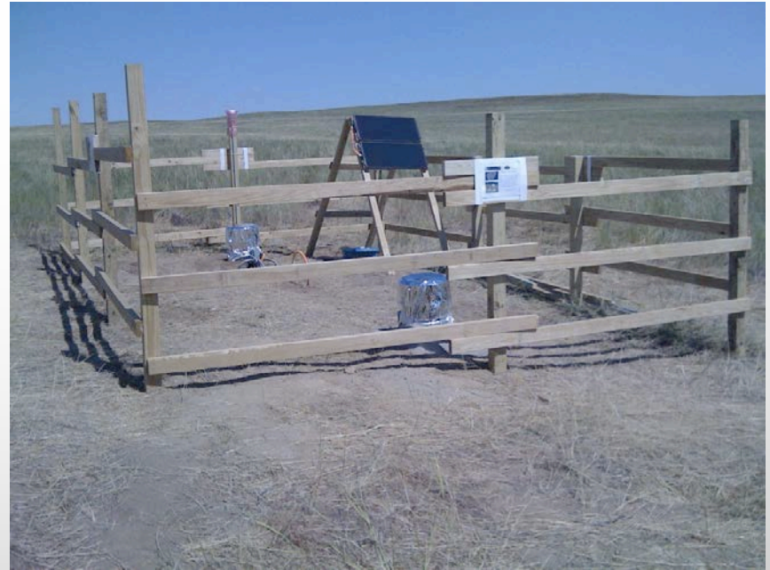
(right) Narod NIMS underground vault observatory with 3G telemetry
