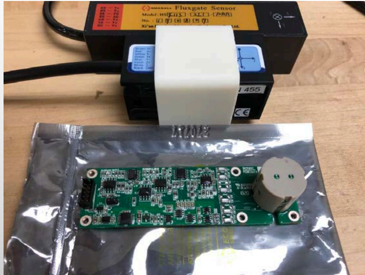
(left) One SMAGALL and two Bartington fluxgates
