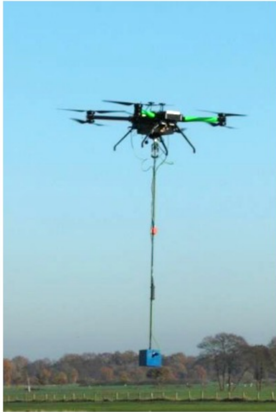
Figure 6: Octocopter. The MTOW is 25 kg. The max payload is 10 kg @ 25 min endurance
