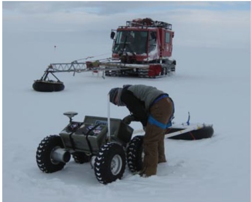
Figure 2. Polar rover Yeti during operations in the McMurdo shear zone, Antarctica, in 2010. Yeti towed the same 400 MHz GPR antenna (located in an inner tube) as pushed ahead of the Pisten Bully manual GPR vehicle (seen in the background). Note the low wheel sinkage, typical for the 81 kg rover on natural polar snowfields.
