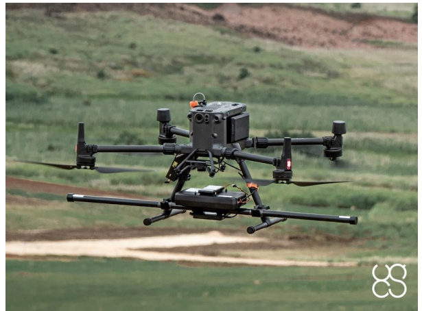
SENSYS MagDrone R3 magnetometer Payload is ~1kg
