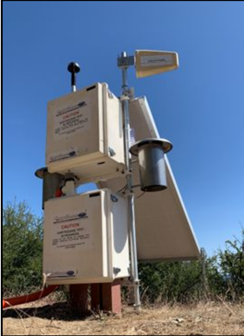
QF Station installation with Solar Panels, and Communications.
