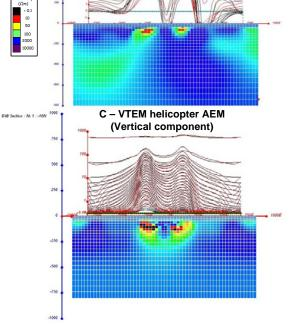
element method (CFEM). The inversion results presented below are for the synthetic data generated from a 1  $\Omega$ m block embedded in a 1000  $\Omega$ m half-space, where the starting model was a uniform 1000  $\Omega$ m half-space.
