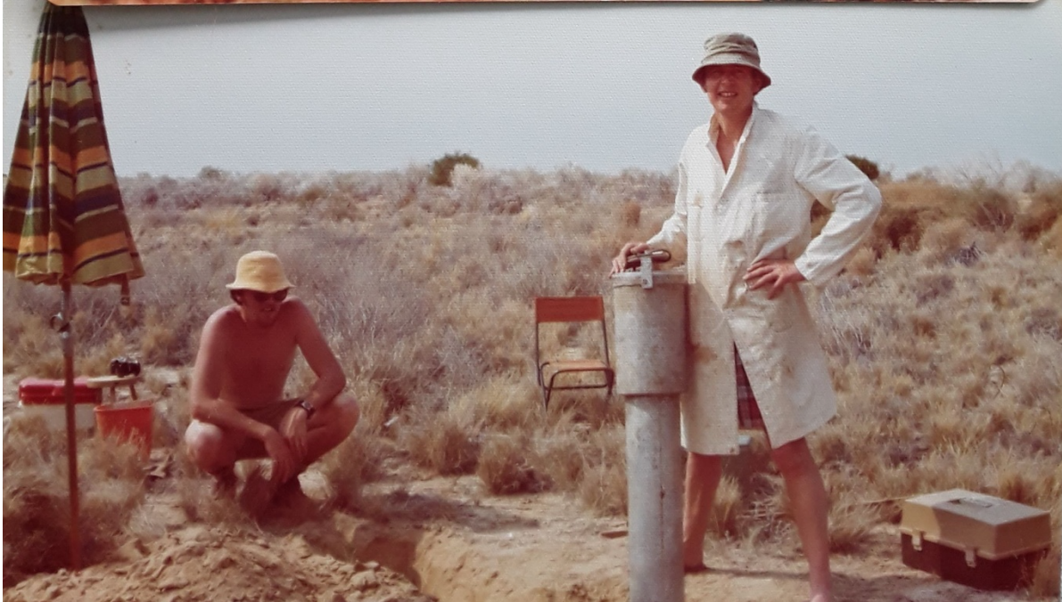
Ted and his able bodied (then anyway) assistant installing a Gough-Reitzel magnetometer. Note Ted, ever the scientist, in his lab coat in the heat, while I'm half naked.
