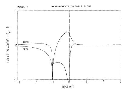
Fig. 8. The inductive response of model 4 represented in terms of the induction arrow. Over the continental shelf the arrow is computed at the ocean floor. The full line corresponds to an extension of model 3, i.e. with a changing lithospheric thickness. The dashed line arises from an extension of model 2. Note the minute difference between the two curves.
