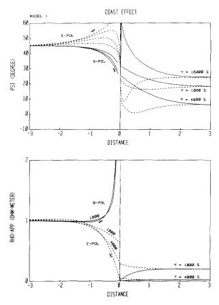
Fig. 2. MT response of model 1. To avoid crowding the graph the curves corresponding to  $\tau = 16000$  S have not always been plotted. We recall that the horizontal distances are given in terms of the skin-depth in lithospheric material. One unit therefore amounts typically to 100 km for material of 100  $\Omega$ m resistivity at a period of  $40\pi^2 \approx 400$  s. The same scale length applies to all the following figures.
