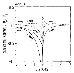
Fig. 7. The inductive response of model 3 represented in terms of the induction arrow. For the sake of clarity the intermediate curve with  $\tau = 4000$  S is left out.
