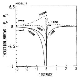
Fig. 6. The inductive response of model represented in terms of the induction arrow. For the sake of clarity the intermediate curve with  $\tau = 4000$  S is left out.
