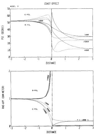
Fig. 4. MT response of model 3. To avoid crowding the graph part of the  $\tau = 16000$  S curve is left out in the apparent resistivity plot.
