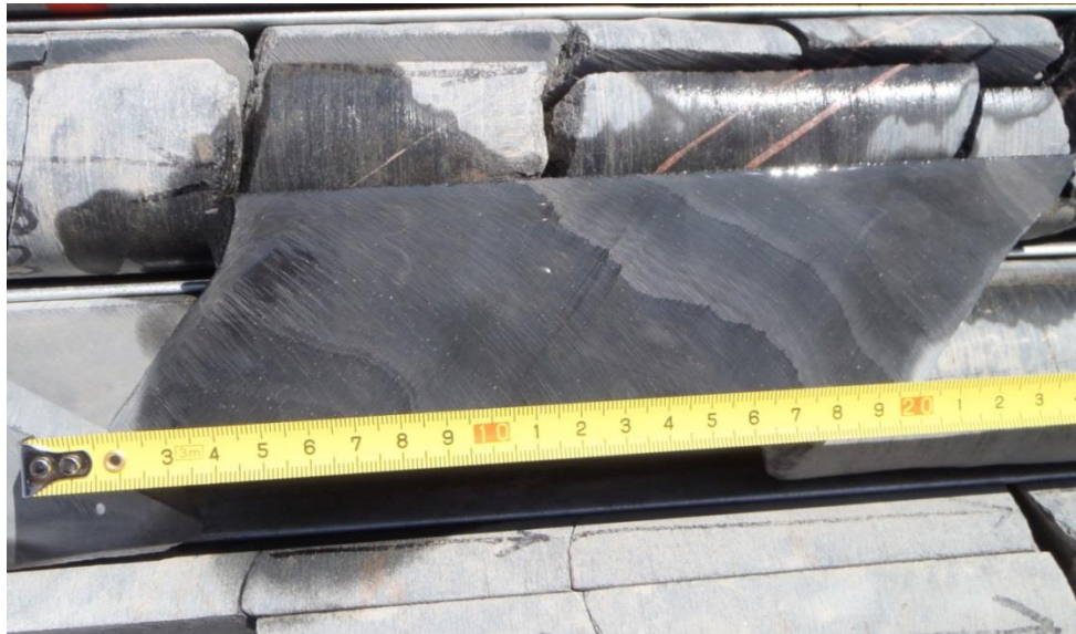
Figure 6.21: Photograph of the low-grade greenschist metamorphism overprinted on shale intersected in borehole 1821C3. Figure 6.22 shows the location of the borehole.
