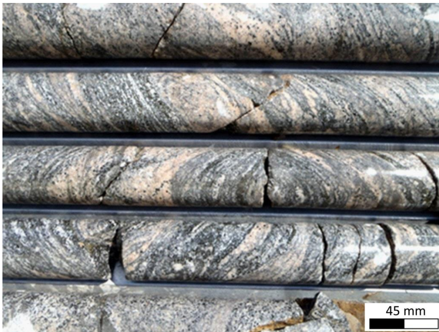
Figure 6.13: Photograph of the typical gneiss intersected in borehole G3. Location of the borehole is shown in Figure 6.12.
